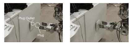
Fig. 14. Adjustment without compli- Fig. 15. Insertion with compliance moance motion tion
