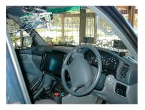
Fig. 4. Inside the ANU/NICTA intelligent vehicle. Cameras to monitor the road scene appear in place of the rear-vision mirror.
