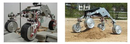
Fig. 3. A four-wheel mobile test bed for initial experiments
