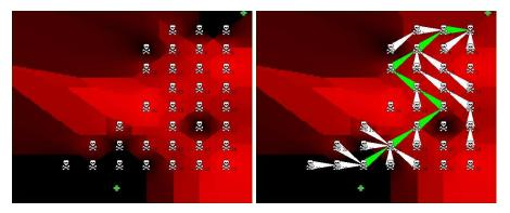
Fig. 5. (Left) Potential field danger map computed by sensors in response to the simulated presence of a chemical agent. (Right) Safest path computed for a trapped first responder by the sensor field.
