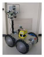
Fig. 4. A four-wheeled rescue robot FUMA with LRF. FUMA has five cameras and one on the top of the arm is used for the experiment. The yellow box on the body of the FUMA is the laser rangefinder, RS4-4 which is used as a positioning sensor.
