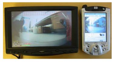
Fig. 2. Example LCD screen tested for lower arm mounting. The contrast is, however, a major challenge for outdoor usage. The screen is shown together with a corresponding iPAQ interface that can be used for portable control, but again with contrast issues
