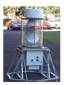
Fig. 5. Outdoor scanning terrain imaging millimeter-wave radar unit
