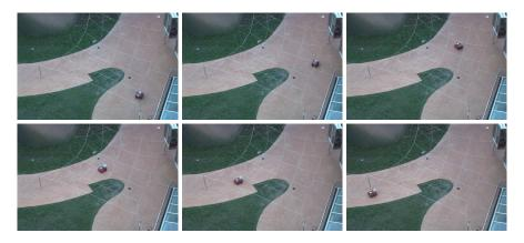
**Fig. 7.** Six snapshots of a guided navigation experiment. The Mica Motes are located as shown in Fig. 6. The optimal node sequence is 2, 3, 4, 9, 13, 16, 19. Because the viewing angle is not directly from above and there is some distortion in the net, the robot does not line up exactly with the node locations.
