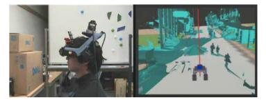
Fig. 10. A snap shot of the developed MR-based teleplesence display (right) that is interactive with the operator's head motion (left)
