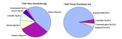
Fig. 6. Mass and power distributions in "OS4" robot.
