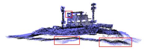
**Fig. 3.** Registration results obtained by considering reference (light blue) and sample (black) to be rigid. The side view reveals, that there remain huge divergences (red boxes) between numerous parts of the two point clouds.
