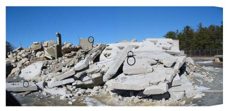
Fig. 1. Wide angle view of sensors placed on rubble. Most of the sensors are behind outcroppings and hence are not visible. The circles show the locations of a few of the sensors.
