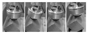
Fig. 16. the sequential photograph of swaying ankle to both sides to detect an edge of a beam or a step
