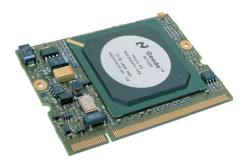
Fig. 3. X-board <861> single board computer from Kontron
