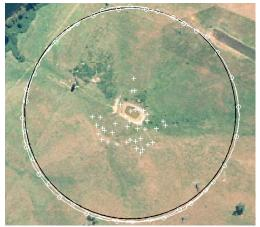
Fig. 11. An orbit around a feature (dam). The desired path (black line, 170 m radius) and navigation solution (white line) are indicated. At 1 second intervals, the position of the FV (white circles), and the projected centre of the sensor frame on the ground (white crosses) are shown.
