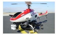
**Fig. 1.** The NASA/ARP helicopter equipped with a range measurement device from SICK.
