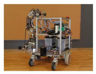
Fig. 3. Target robot (Autonomous mobile manipulator)
