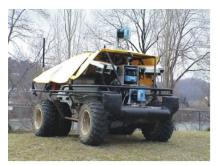
Fig. 1. The PerceptOR off-road mobile robot. The experiments were performed with this and similar vehicles.
