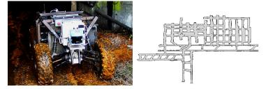
Fig. 1. Left: Groundhog, the current robotic platform of the mine mapping project. Right: This map was generated from data acquired during experimentation and utilizes offline globally consistent mapping techniques. It shows the highly cyclic nature of room-and-pillar mines.
