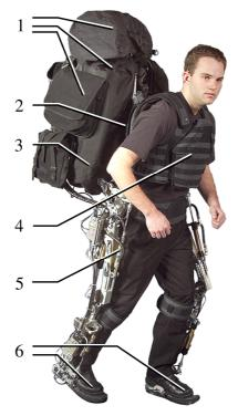
Fig. 1. Berkeley Lower Extremity Exoskeleton (BLEEX) and pilot Ryan Steger. 1: Load occupies the upper portion of the backpack and around the Power Unit; 2: Rigid connection of the BLEEX spine to the pilot's vest; 3: Power unit and central computer occupies the lower portion of the backpack; 4: Semirigid vest connecting BLEEX to the pilot; 5: One of the hydraulic actuators; 6: Rigid connection of the BLEEX feet to the pilot's boots. More photographs can be found at http://bleex.me.berkeley.edu
